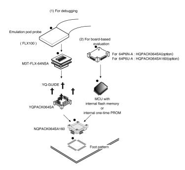
•: position of No. 1 pin. Be sure to match the position of No. 1 pin of the foot pattern and each part.
